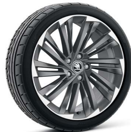
19" kola z lehké slitiny Veritate antracitová disk: 8J × 19" ET44 pneu: 235/40 R19
